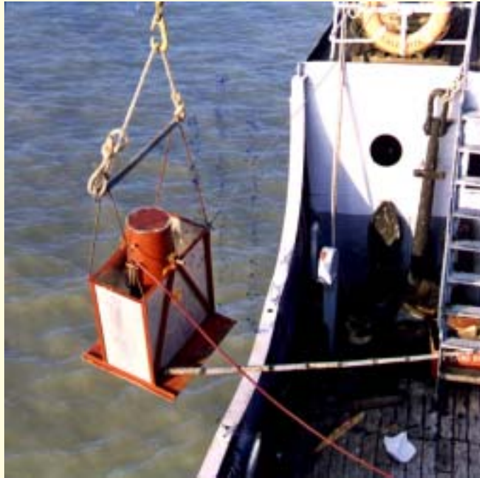
Radiotracer studies being conducted in Hoogly river to study silt movement. Below: Radioisotopes being used to determine mercury inventory in electrolytic cells
