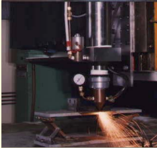
Laser cutting mild steel plate developed at CAT
