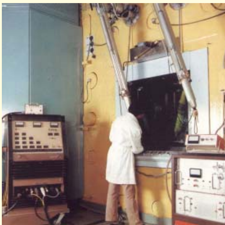
At BARC: Hot Cell facility for production of radioisotopes
