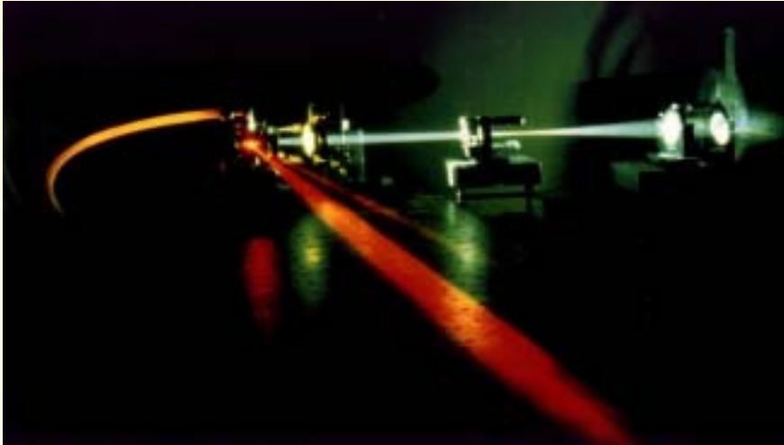
Dye-Laser Pumped Copper Vapour Laser. Both these lasers were developed and fabricated inhouse
