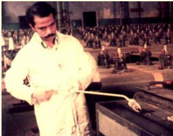
Radiotracer studies being conducted in Hoogly river to study silt movement. Below: Radioisotopes being used to determine mercury inventory in electrolytic cells
