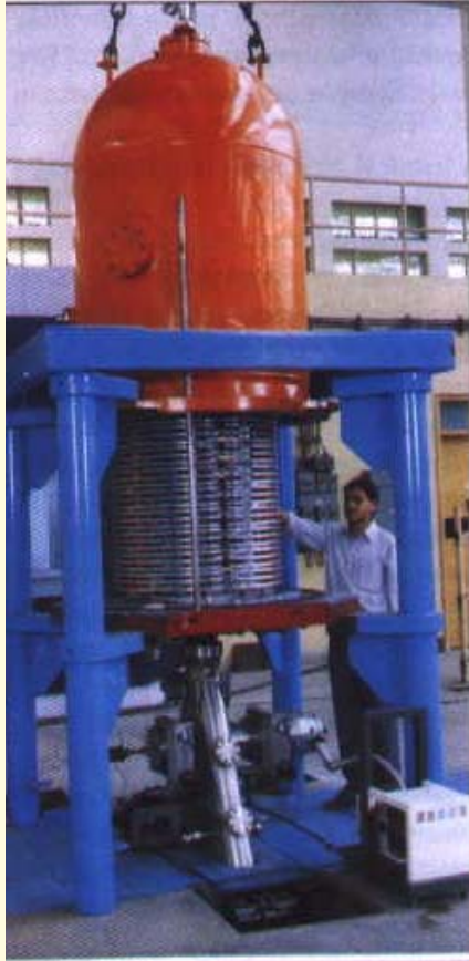
500 keV Electron Beam Industrial Accelerator of BARC installed at Vashi, Navi Mumbai for various radiation processing applications. (Left) Radiotracer studies at a trickle bed reactor in a factory
