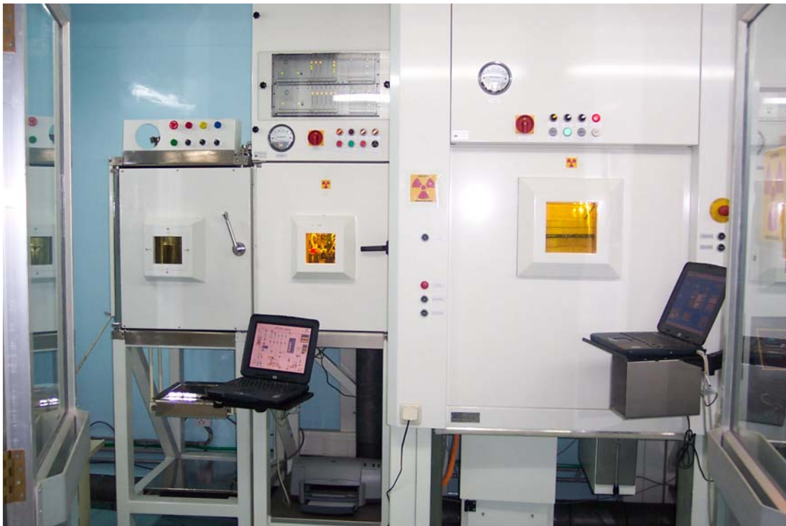
Fully programmable chemistry modules and dispenser used for the synthesis and sterile dispensing of injectable PET radiopharmaceuticals
