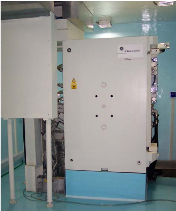
The medical cyclotron facility for the production of short lived positron emitting radionuclides
