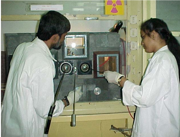
A shielded facility for the production of iodine-131 capsules for therapeutic applications
