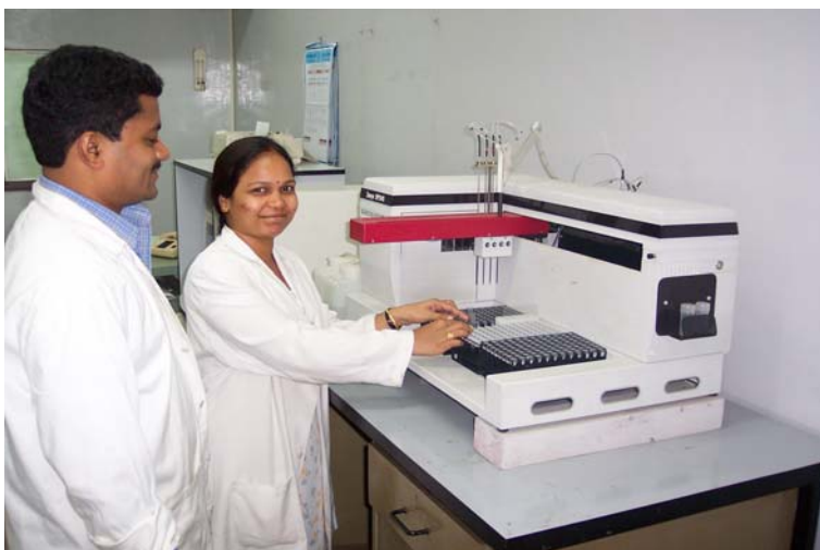
Robotic sample processor for RIA/IRMA that can process samples automatically
