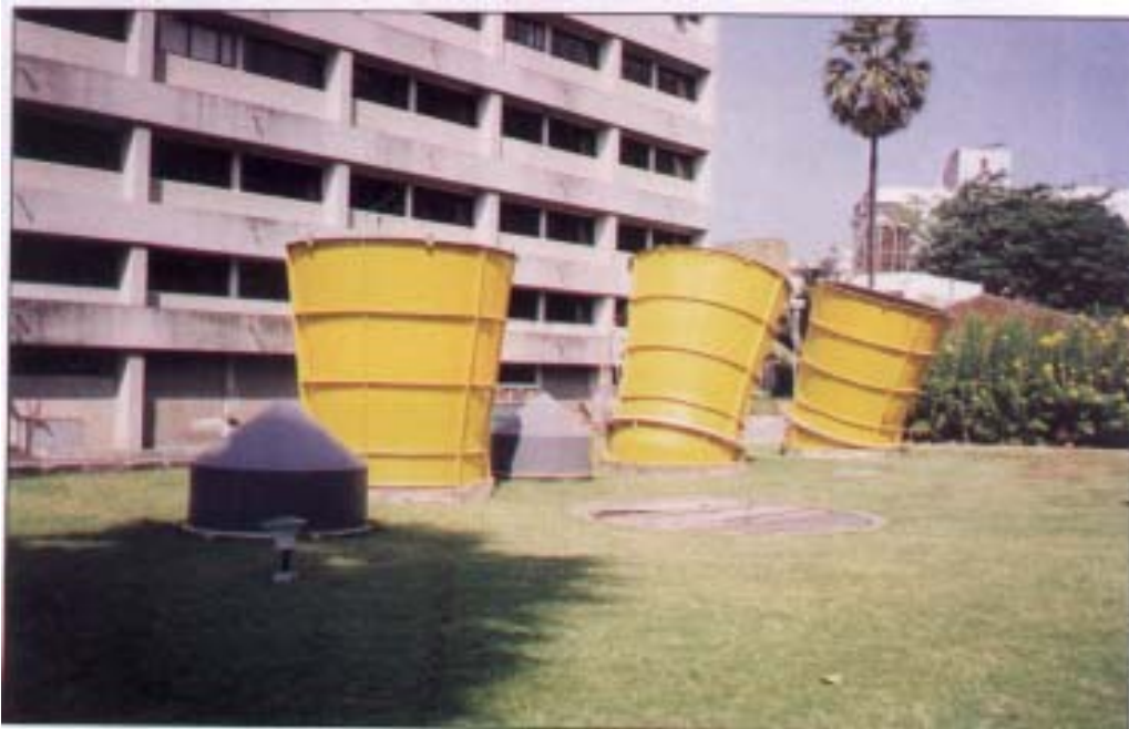
Doppler SODAR (Sound Detection and Ranging) system. BARC collaborated with SAMEER, Mumbai for this development work.
