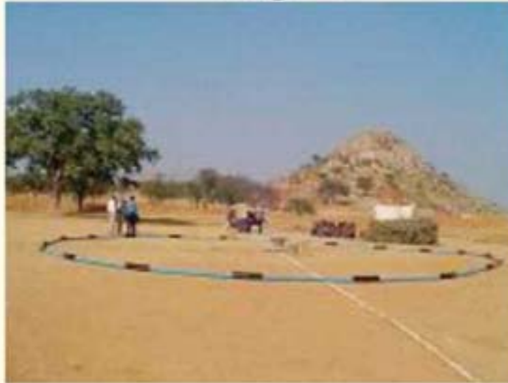
Figure 16: Time Domain Electro Magnetic System being tested at Rohil, Rajasthan
