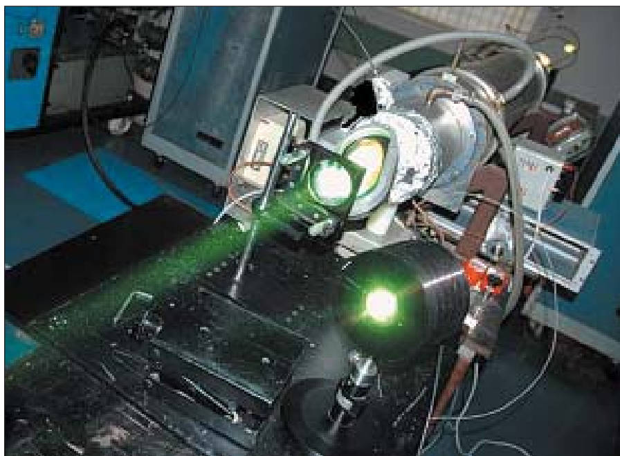
100 Watt kinetically enhanced copper vapour laser developed at RRCAT
