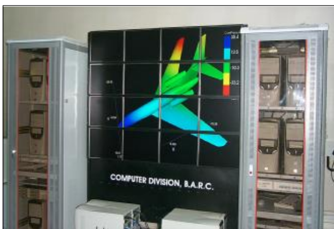
A postprocessor (AnuVI) supporting large tiled display graphics cluster for visualization of data generated in Computational Fluid Dynamics applications
