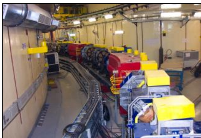
A view of part of the 172m circumference, 2.5 GeV electron Indus-2 storage ring
