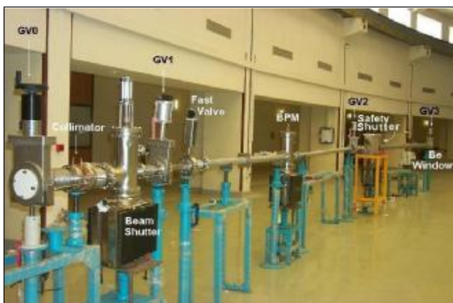
Prototype front end assembled in the Indus-2 experimental hall
