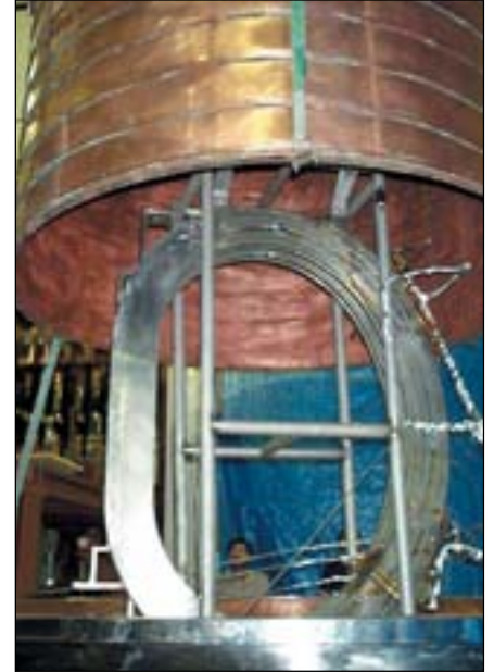
Superconducting TF coils under test
