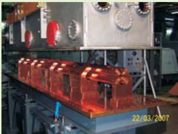
Fig. 4. 3.4 m long Radio Frequency Quadrupole accelerator during assembly
