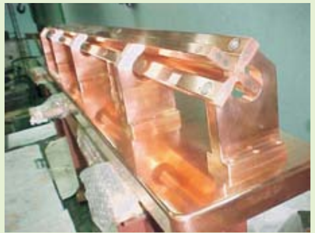
Fig. 3. 1.7 m long Radio Frequency Quadrupole accelerator during assembly
