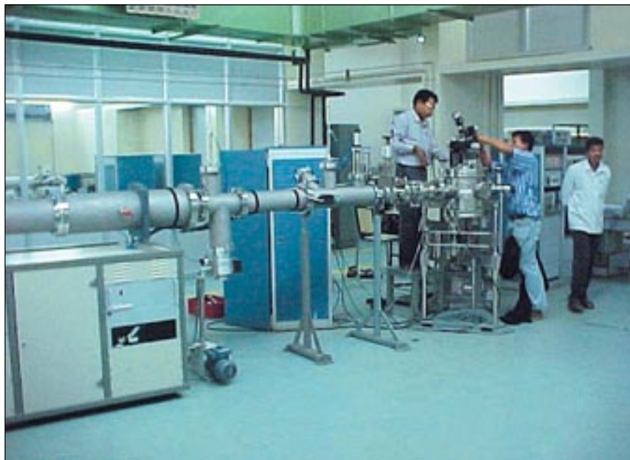
The 1.7 mega volt Tandetron Accelerator at the Materials Science Division, IGCAR.. This accelerator is being used for experiments on simulation of radiation damage using ion beams, synthesis of novel phases by irradiation and materials characterization using Rutherford backscattering, channeling and PIXE. The accelerator facilities at IGCAR are extensively used by the students under the UGC-DAE-CSR programme.
